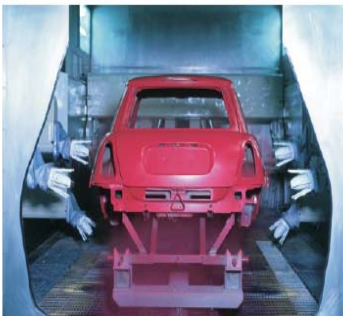
Figure 5. Automated spray painting of a car body in a BMW plant
